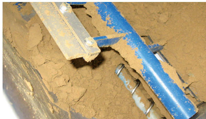
Agitator for product activation and fluidisation
