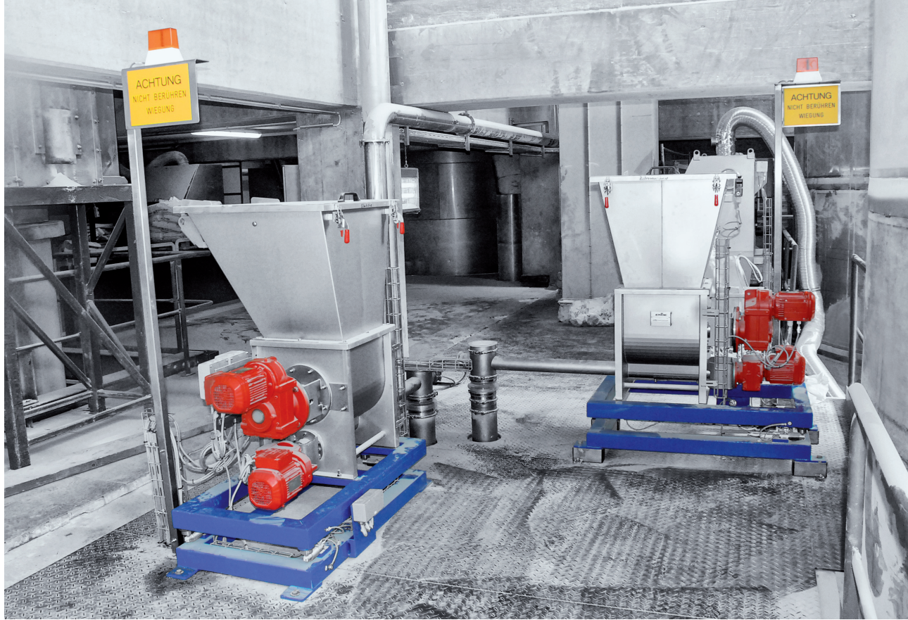
Gravimetrically controlled batch dosing in the salt industry
