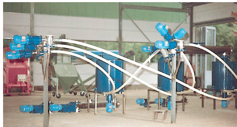
Flexible spiral conveyors fitted for FAT test
