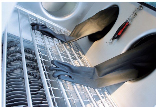
Sack discharge cabinet with downstream lump crusher
