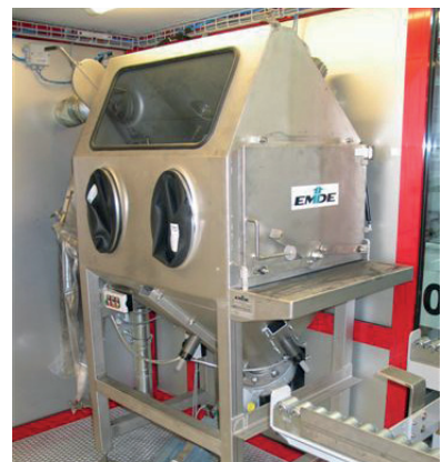
Sack discharge cabinet for handling soot
