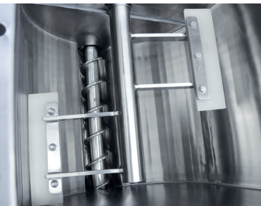
Dispersing agitator with exchangeable PU paddle
