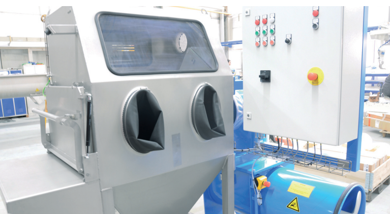
Feeding door with tightly closing flap
