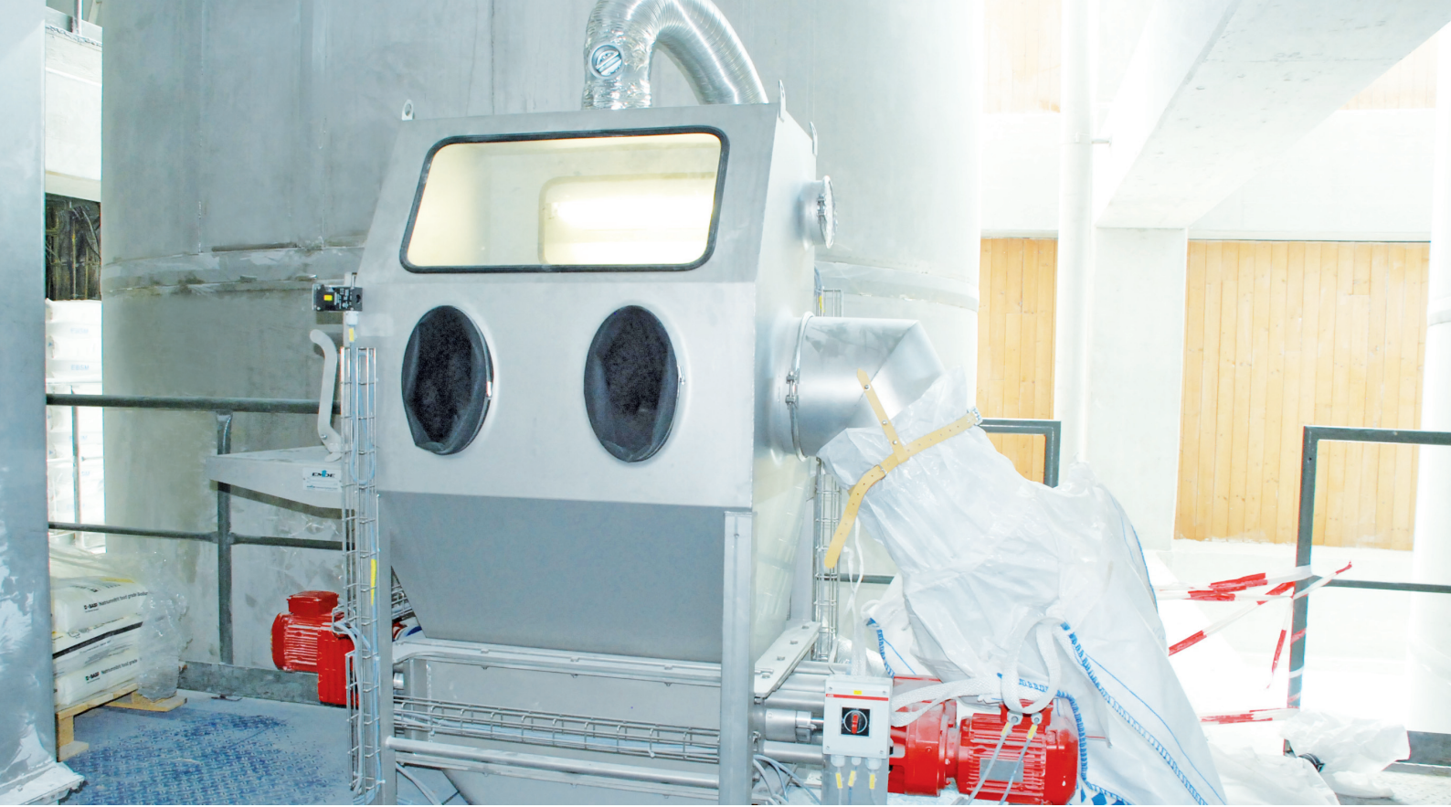
Sack discharge cabinet used in the salt industry
