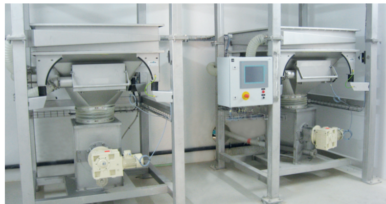
3 Big Bag emptying station with connected EMDE-LIFT
