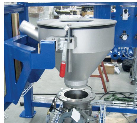
30 Docking plate with hand lever tighteners
