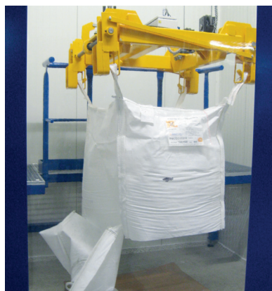
36 Big Bag bottom sliced open on 3 sides
