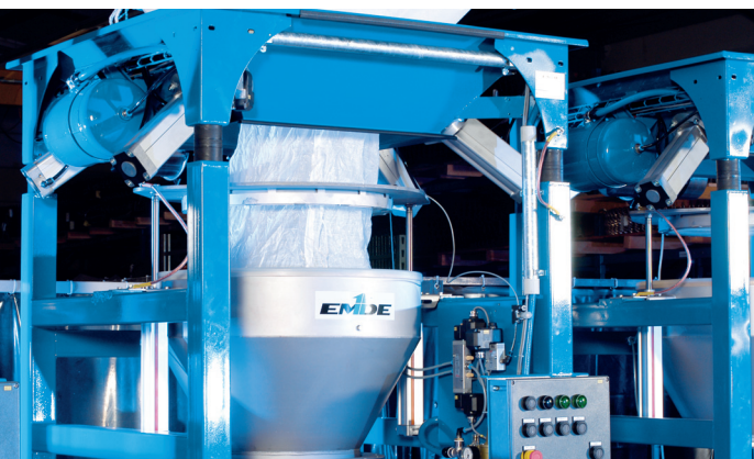
28 Dust proof connection discharge spout Big Bag
