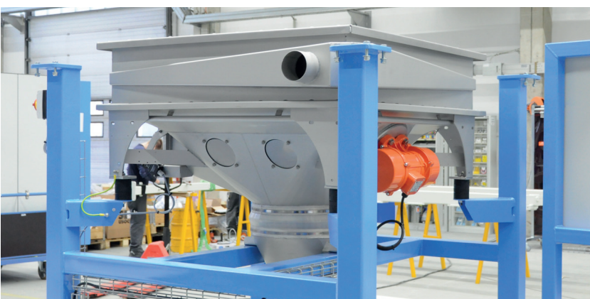
25 Type BE 1500 with dust aspiration duct
