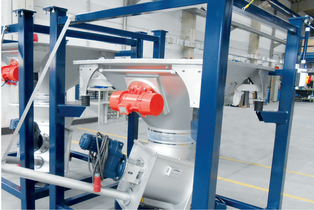
20 Big Bag emptying station with vibration discharge bottom and downstream metering screw
