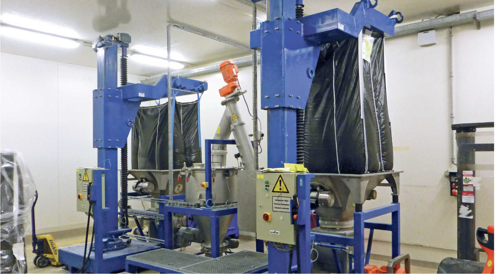
24 Big Bag emptying station type BE 1500 HSS with lift/swiveling column
