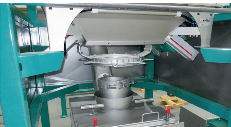
32 Type BE 1400 with discharge lock system
