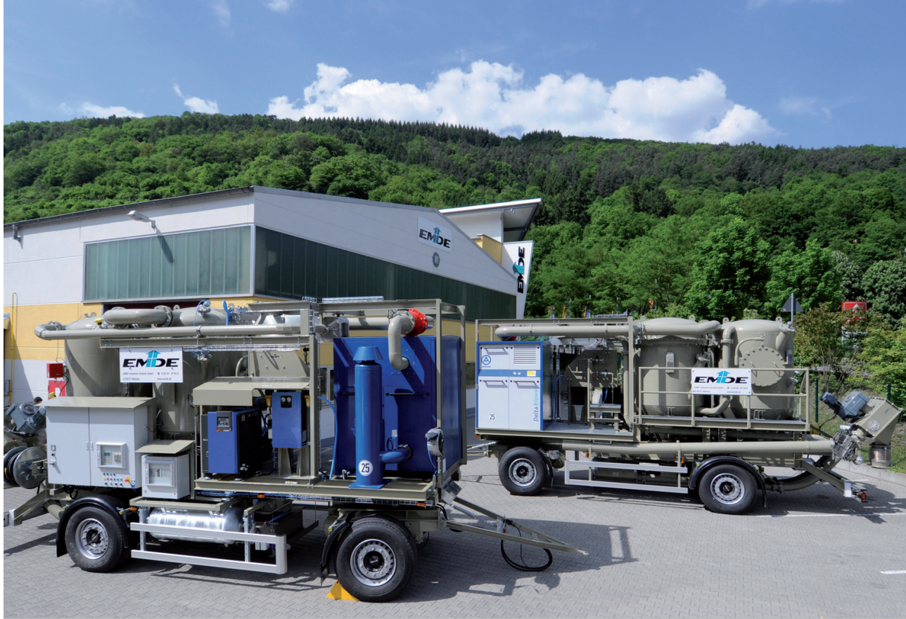
Antisurge protection system with pre-cleaner and filter separator
