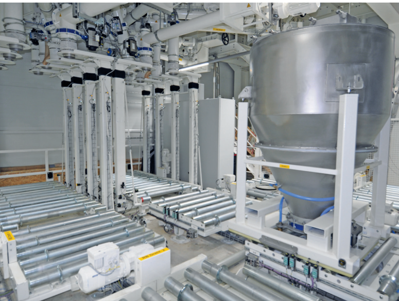
Transport via robust roller conveyor system with turntable
