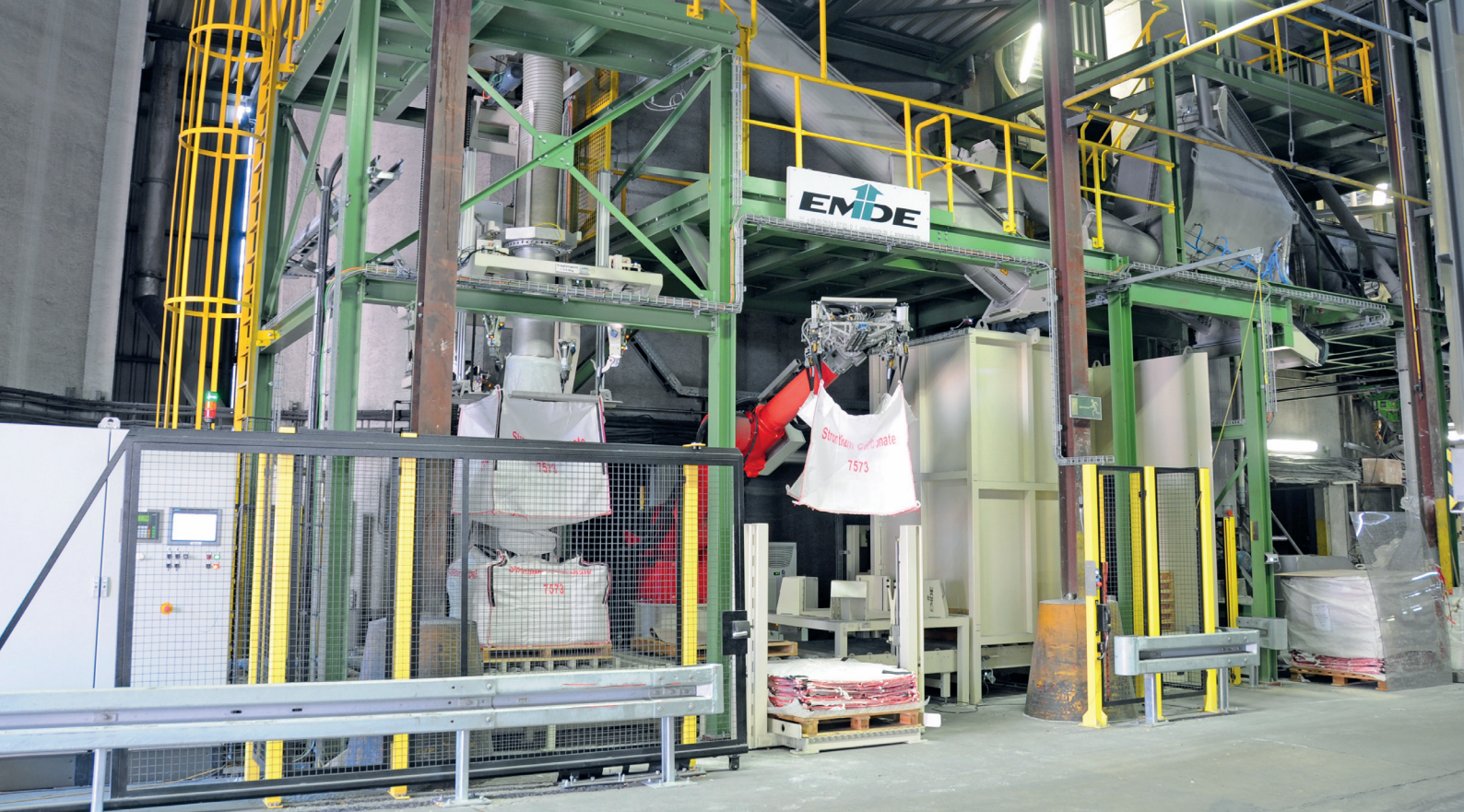
Complete system with product dosing via screw conveyor
