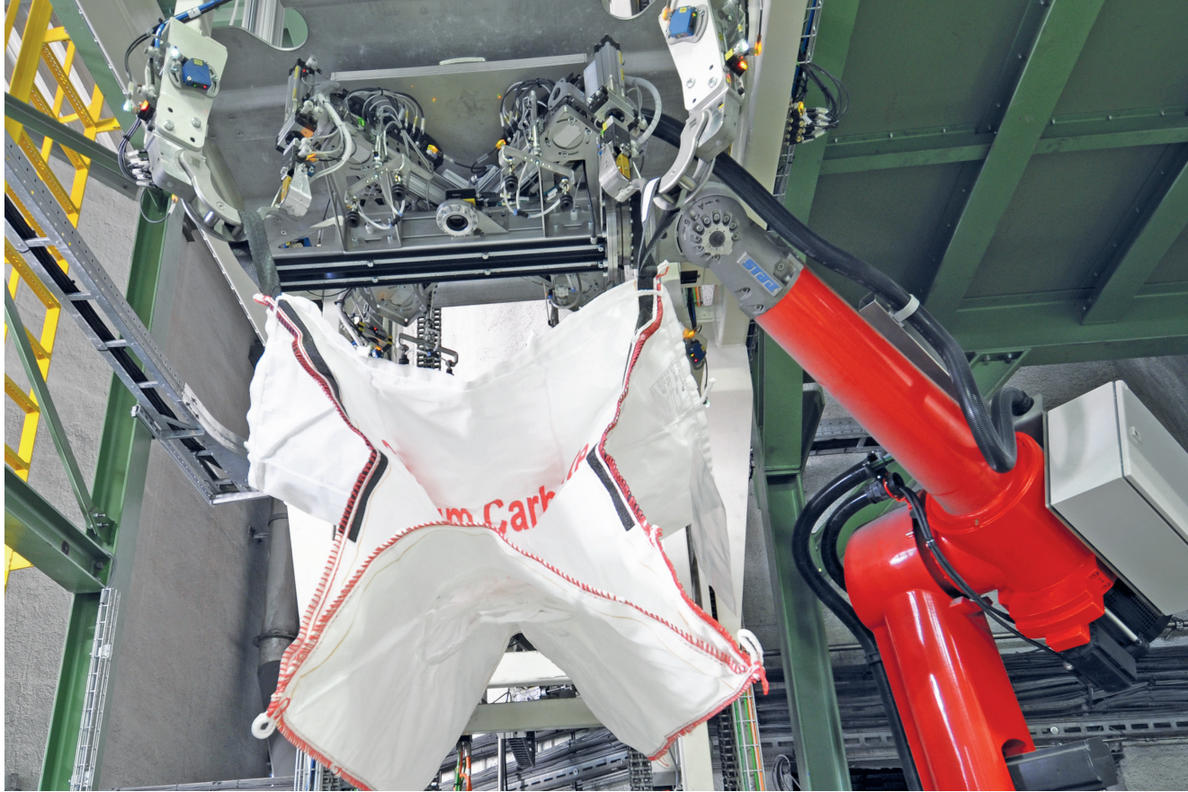
Robot controlled Big Bag transfer in filling station
