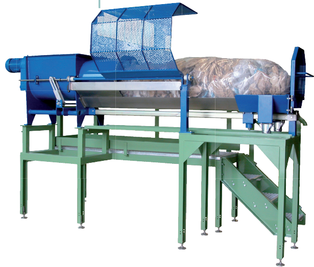
Empty Bag Compactor with automatic brake slide relief
