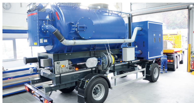
Mobile vacuum cleaning system for ash
