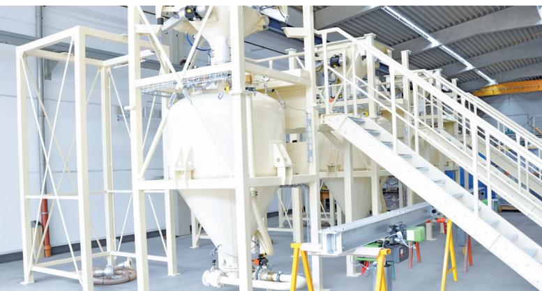
Pressure bin conveying system assembled for FAT
