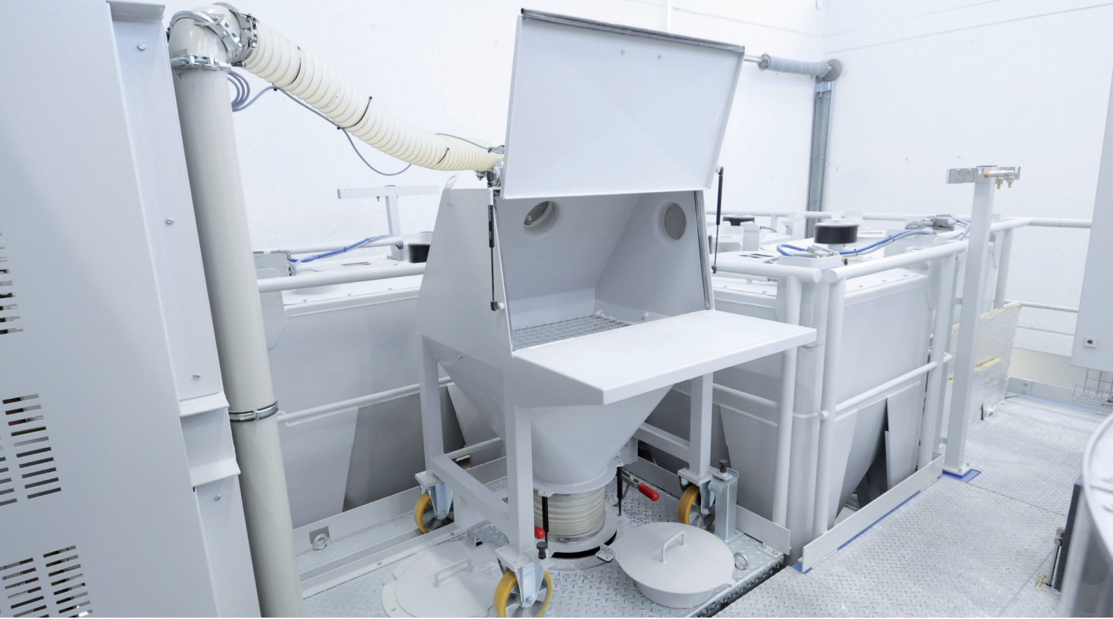
Sack chute with discharge docking
