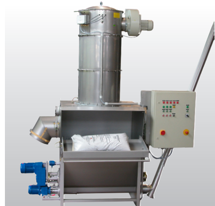
Emptying sacks with force feeder/steep screw conveyor
