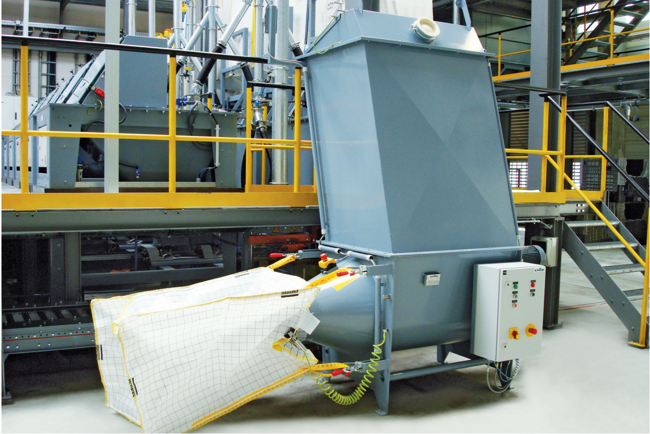
Big bag compressor with extended insertion chute
