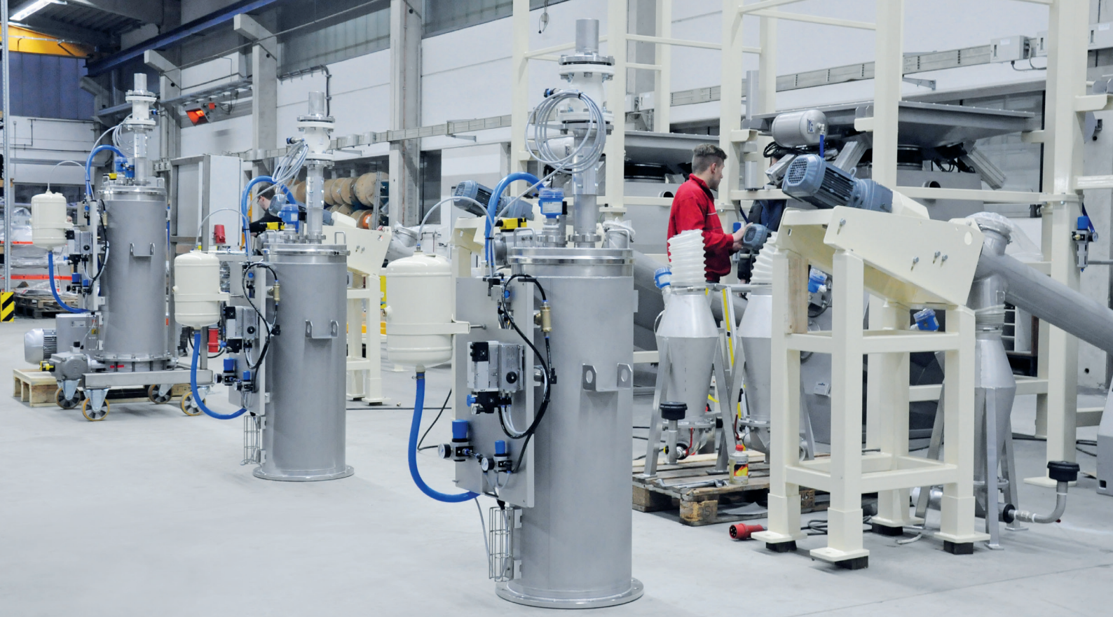
Vacuum conveyor in final assembly
