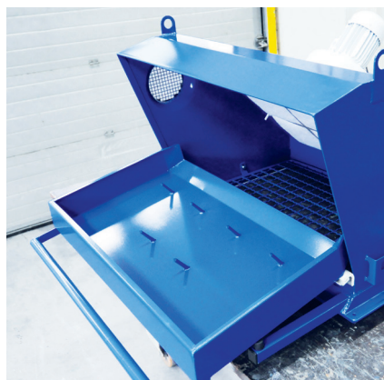
Sack discharge with holding spikes to fix sacks
