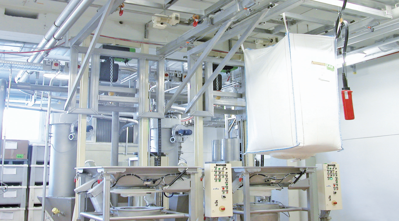
Big Bag emptying station with movable carrying frame
